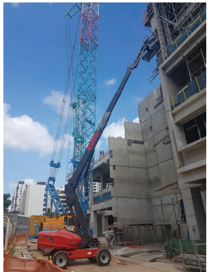
The 260 TJ-X features an offset of 19.7 m, pendulum travel of +/-70°, and capacity for continuous 360° rotation of the turret.
