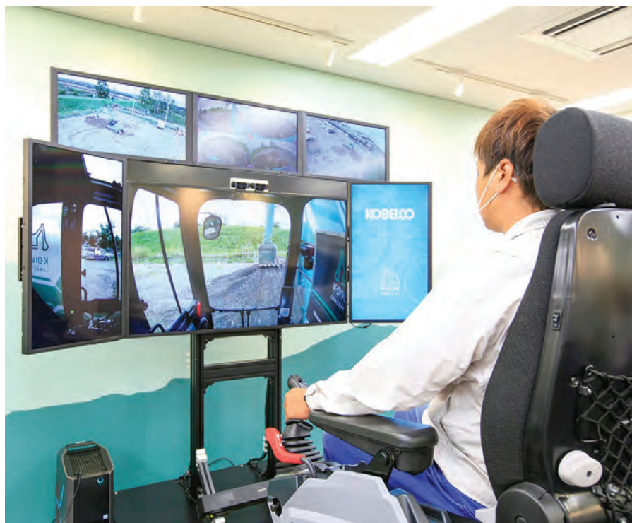
K-Dive Concept is a construction equipment telework service system being developed by Kobelco Construction Machinery, which allows operators to control their excavators remotely without going to the real jobsite.
