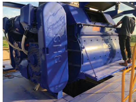
ABOVE: The concrete batching plant with the DKXS 4.00 twin-shaft batch mixer from BHS-Sonthofen produced 18,000 cu m of concrete.
