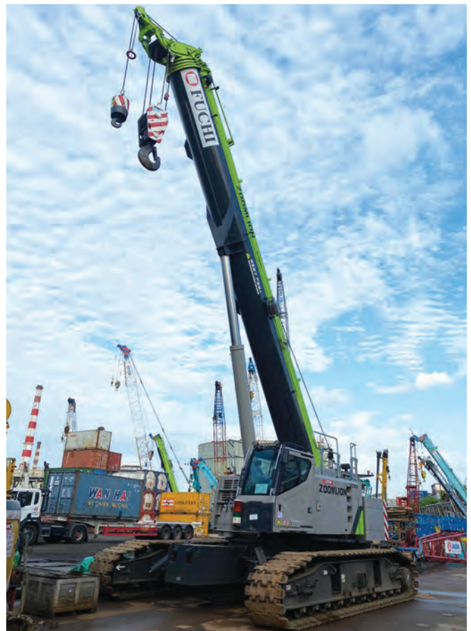
The Zoomlion ZCT900 telescopic crawler crane has a five-section, U-shaped 47-m main boom. It can be equipped with a 14.2-m fly jib to bring the total boom length to 61.2 m.
