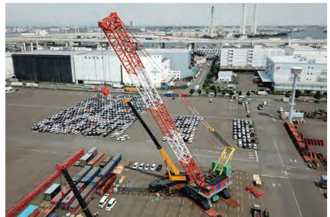
ABOVE AND LEFT: The new Demag CC 8800-1 crawler crane for MIC Co Ltd, featuring an eye-catching paint scheme, will be used in a variety of infrastructure projects such as bridges, steelworks and oil refineries, as well as for the construction of offshore wind power facilities.
