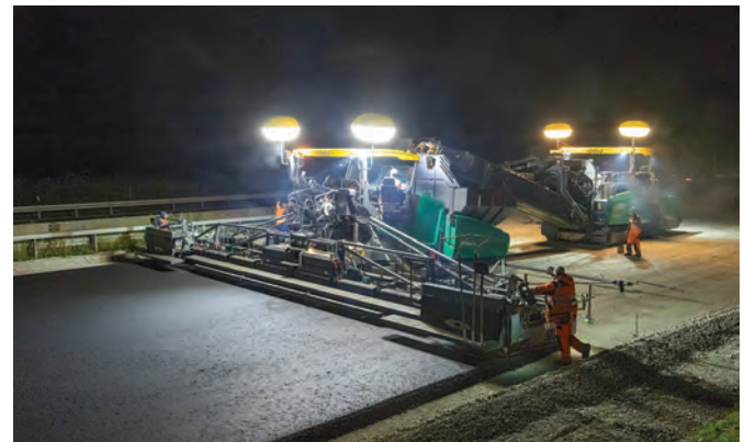
TOP, MIDDLE AND ABOVE: Combined with the SB 350 fixed-width screed, the Super 3000-3(i) paver can deliver a pave width of up to 18 m. The machine is part of the Premium Line from Vögele.
