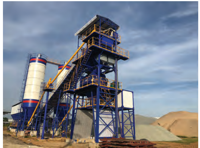
ABOVE: The concrete batching plant with the DKXS 4.00 twin-shaft batch mixer from BHS-Sonthofen produced 18,000 cu m of concrete.
