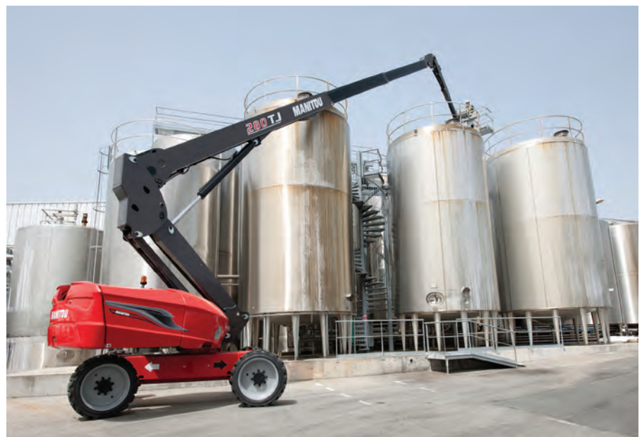
TOP LEFT AND ABOVE: The 280 TJ-X model can rise to a height of 28 m, offering a basket capacity of 350 kg. The machine's continuous turret rotation and working offset of more than 21 m facilitate a wide range of movements without having to move the platform.
