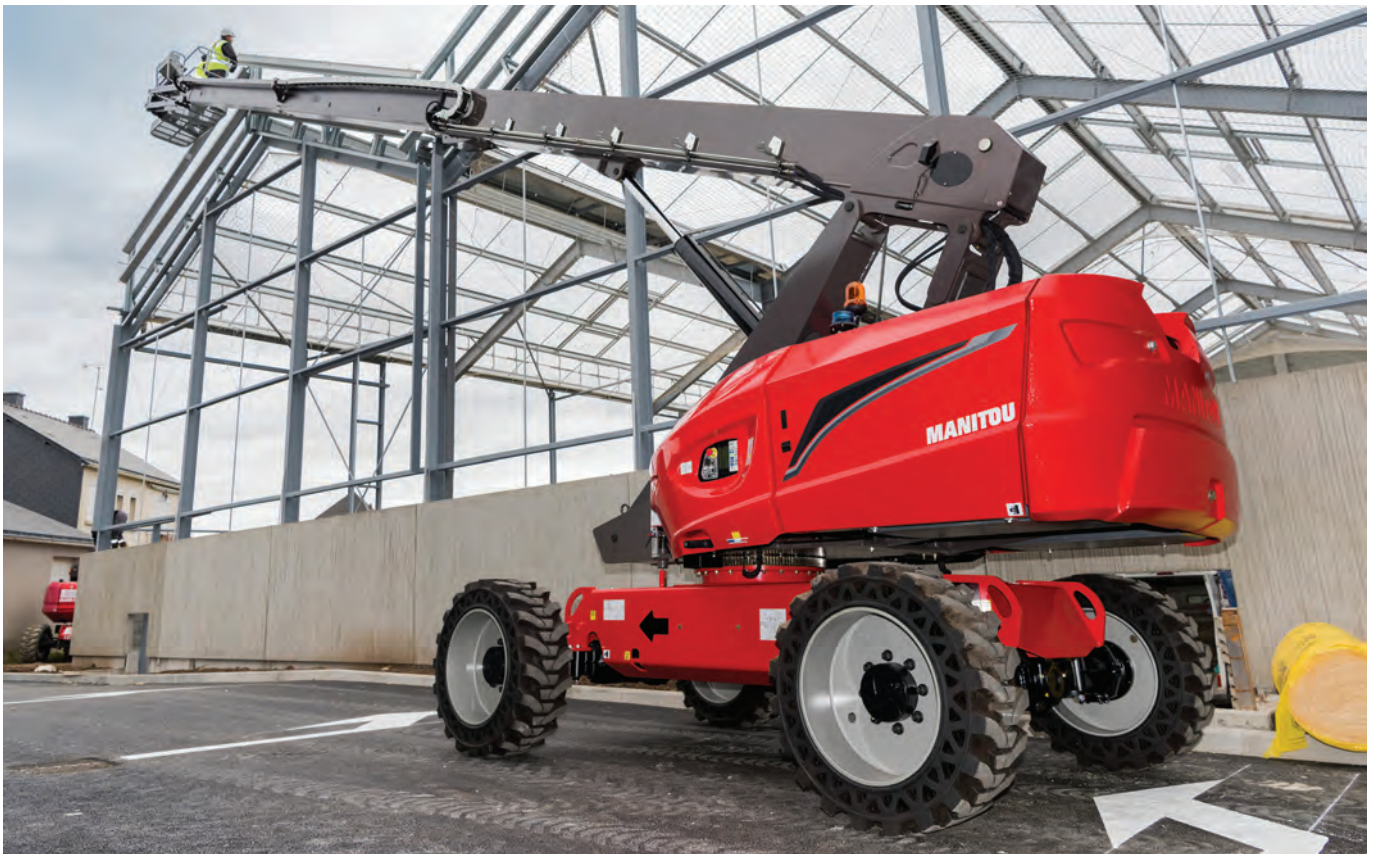
TOP AND ABOVE: The 220 TJ-X and 220 TJ+-X models are capable of reaching a height of 22 m, with a basket capacity of 230 kg and 350 kg respectively.
