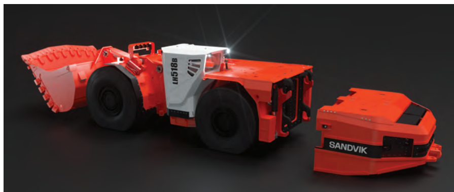
The Sandvik LH518B has been designed entirely around the loader's Artisan battery system and electric driveline.
